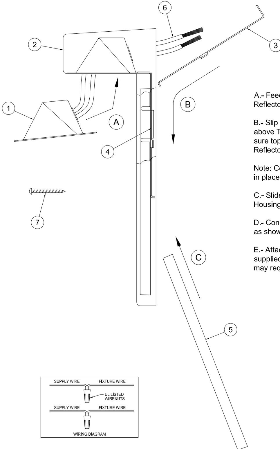
A.- Feed wires through Housing (2) and lift Reflector (1) up into Housing.
